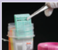
As a cassette holder, the 40 ml HistoTainer™ M960-40MA containing 20 ml of 10% Formalin, is the ideal size container to transport up to four tissue samples pre-inserted in processing / embedding cassettes.
