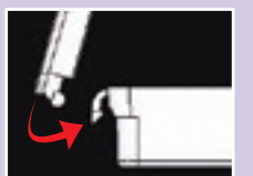
M517-M518 Series The special hinge makes it easy to attach lid to base.
