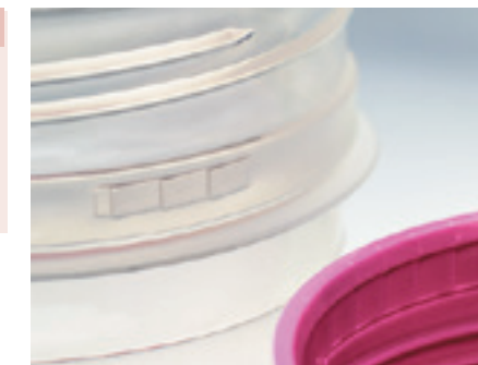
Screw cap on until a clicking noise is heard. This is when the plastic ring is firmly seated and locked over the container threads. When removing the tamper evident screw cap for the first time, the perforation is severed, thereby ensuring easy recognition that the container has been opened.
